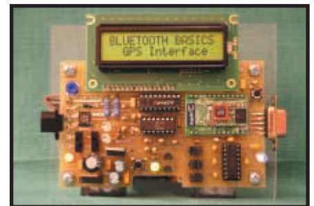
Photo 1 —Take a look at the PIC16F88-based Bluetooth GPS platform. A Wintec WBTV42-D-SPP Bluetooth module sits to the right of the PIC16F88 Nemesis and above the RS-232 interface MAX232 chip. The project wirelessly connects to a GPS module and displays date and time, speed and heading, and latitude and longitude data.
