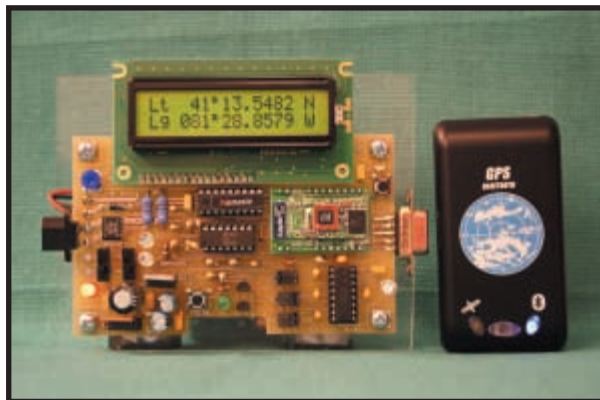
Photo 2 —After first establishing a Bluetooth connection to a GPS receiver, the current latitude and longitude are available for display. The 16-channel Bluetooth GPS receiver provides the data.
